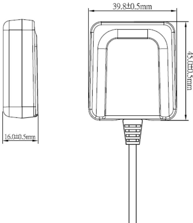
The dimension of GR-701 is 40 mm (W) x 45 mm (L) x 16 mm (H) as shown above.
