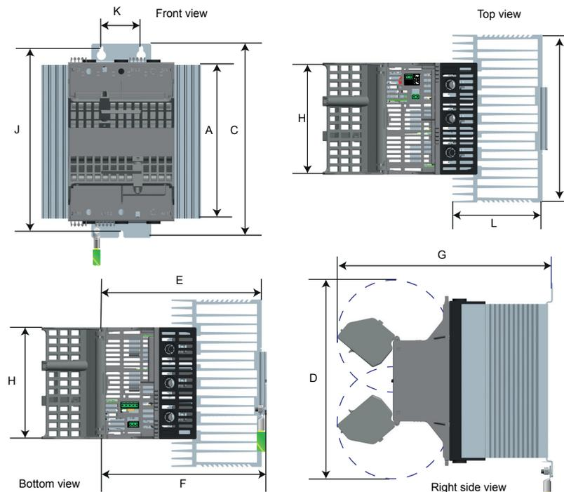
Table 3 Dimensions for EPackLites of different current ratings (all values in millimetres)
