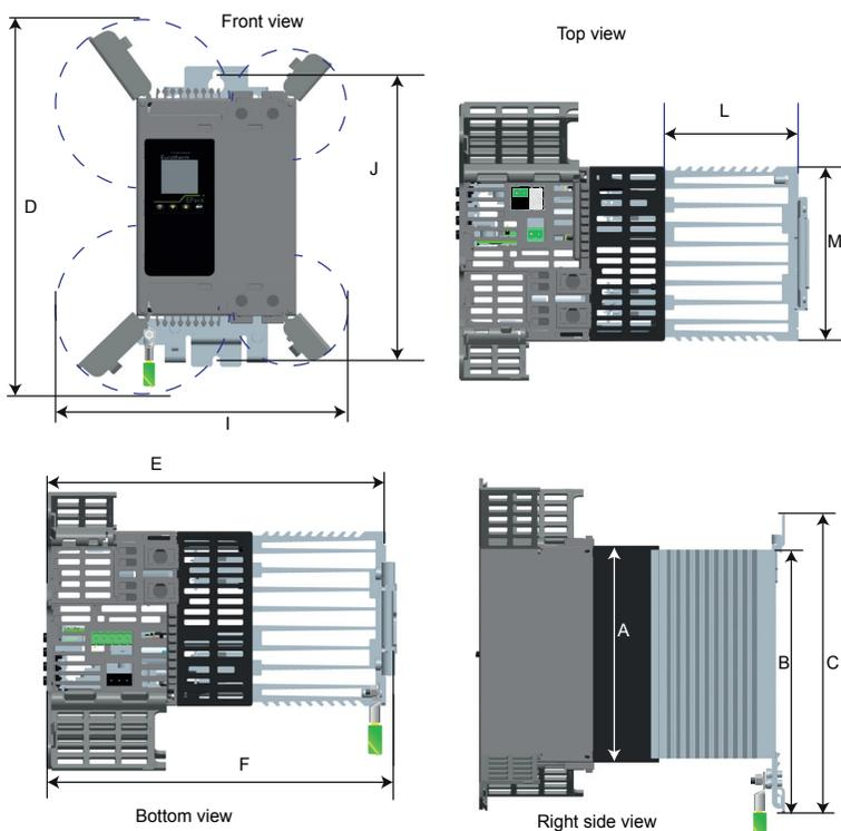
The diagram below shows a 125A EPackLite (doors open), 80 and 100A units are similar— refer to Table 3 for dimensions.
