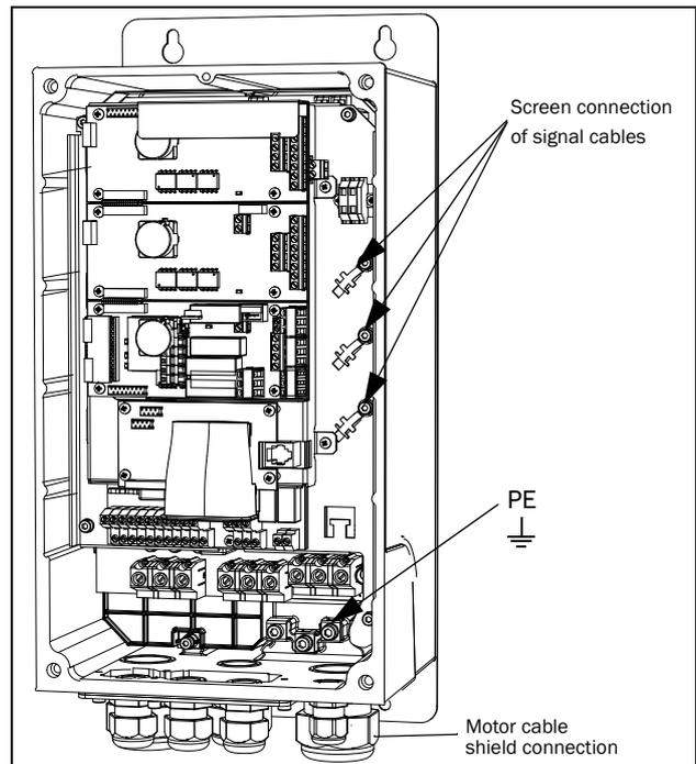
Fig. 32 Screen connection of cables.
