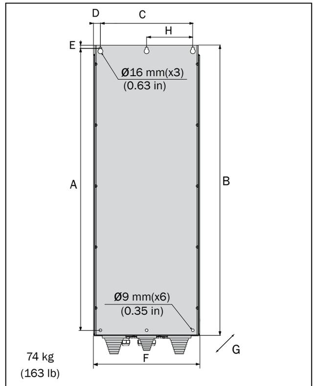
Fig. 17 Emotron FLD Model 48-210 to 295 (Frame size F)
