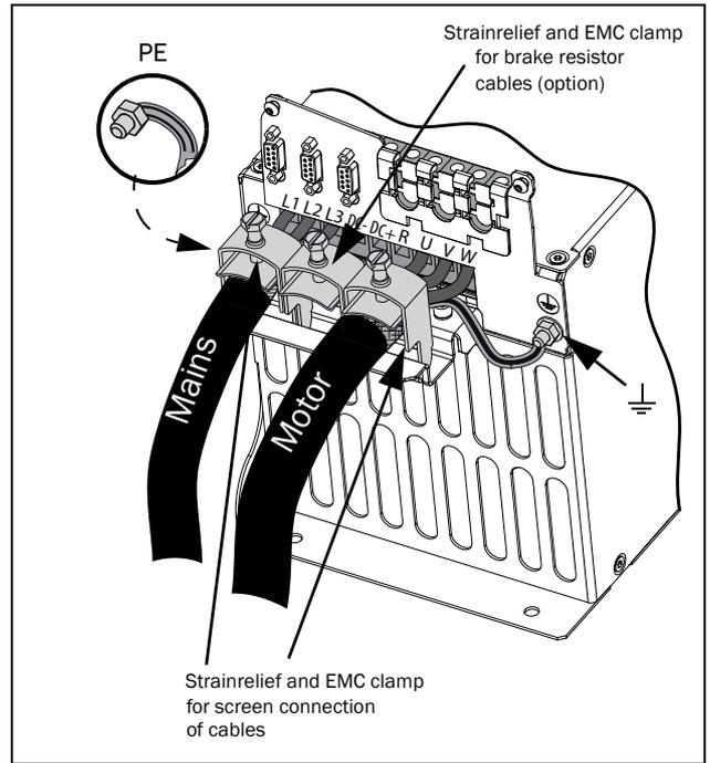
Fig. 26 Mains and motor connections model 48-025 to 48-058, frame size C2.
