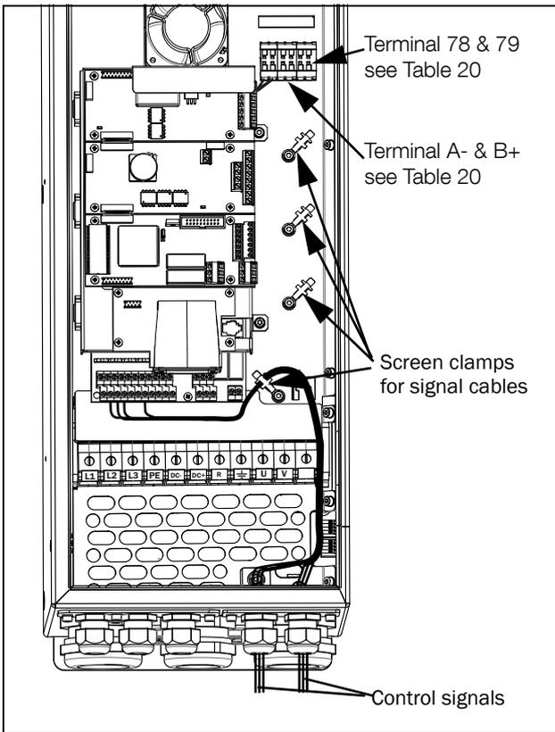
Fig. 45 Connecting the control signals, FLD model 061 to 074, frame size D.
