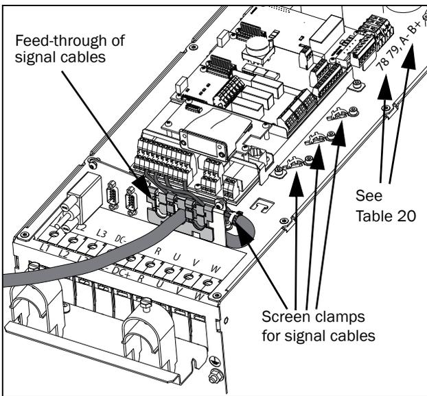
Fig. 46 Connecting the control signals, FLD model 48-072 to 48-105 frame size D2.
