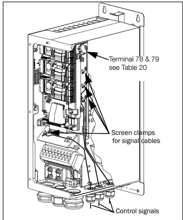
Fig. 43 Connecting the control signals, FLD model 026 to 046, frame size C.
