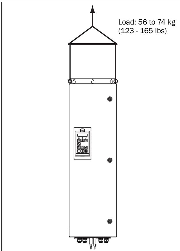
Fig. 2 Lifting AC drive model -090 to -250
