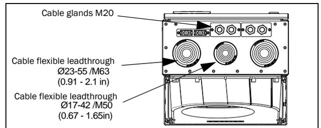
Fig. 18 Cable interface for mains, motor, DC+/DC-, brake resistor and communication, Emotron FLD Model 48-210 to 295 Emotron FLD Model 69-090 to 200.
