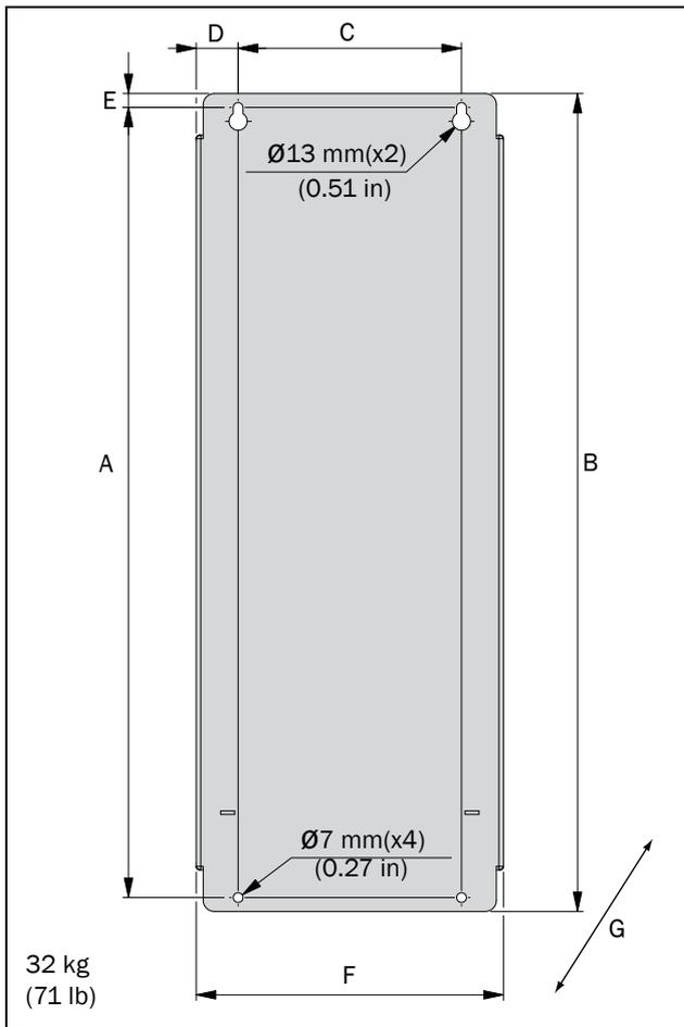
Fig. 11 Emotron FLD Model 48/52-061 and 074 (Frame size D)
