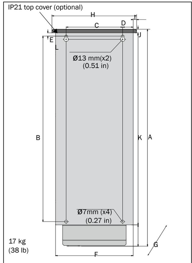
Fig. 9 Emotron FLD Model 48-025 to 48-058 (Frame size C2), backside view.
