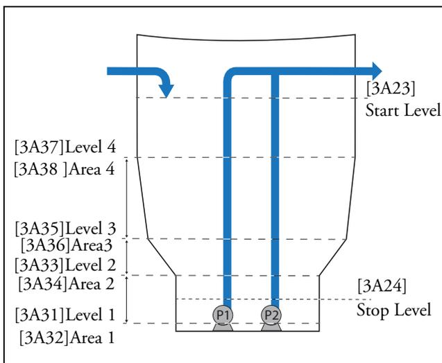
Fig. 54 With this shape, 4 levels and areas are required.
