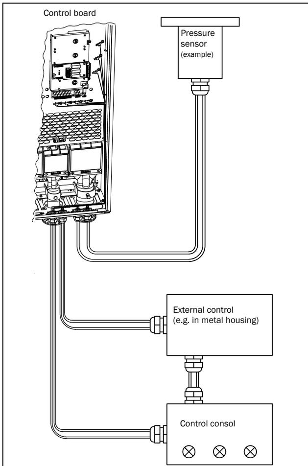
Fig. 49 Electro Magnetic (EM) screening of control signal cables.
