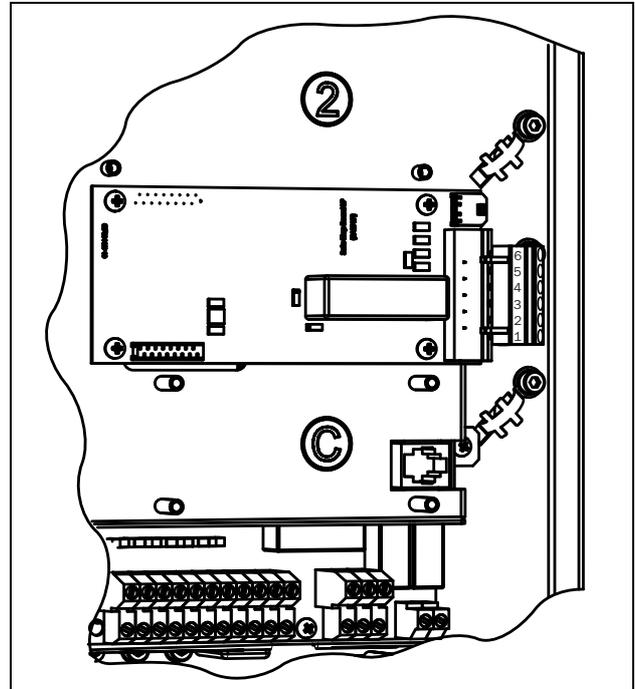
Fig. 58 Connection of safe stop option in size B.
