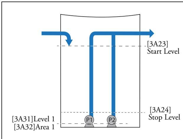
Fig. 53 With a uniform shape, only one level /area is required as the area is the same.
