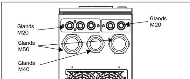
Fig. 12 Cable interface for mains, motor and communication, Emotron FLD Model 48/52-061 and 074 (Frame size D).
