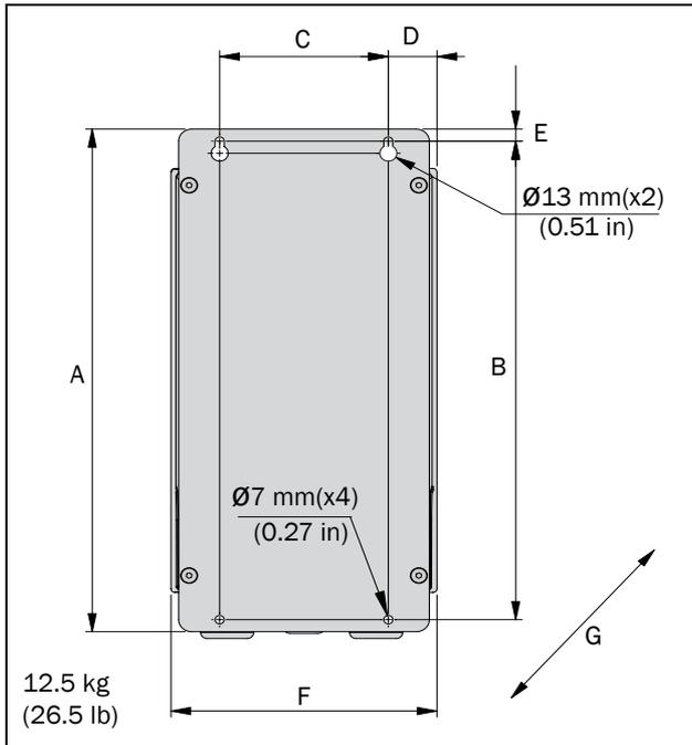
Fig. 4 Emotron FLD Model 48/52-003 to 018 (Frame size B)
