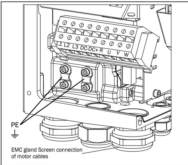
Fig. 25 Mains and motor connections, model 026-046, frame size C
