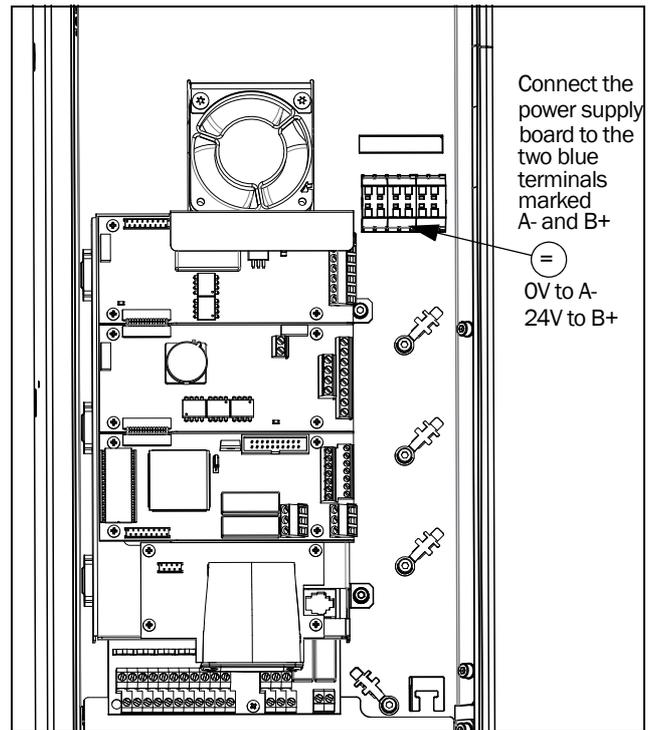
Fig. 57 Connection of standby supply option on frame size D and D2
