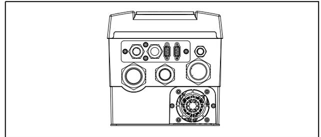
Fig. 6 Emotron FLD Model 48/52-003 to 018 (Frame size B) example with optional CRIO interface and D-sub connectors.
