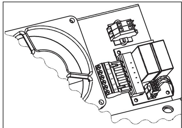
Fig. 59 Connection of safe stop option in size E and up.
