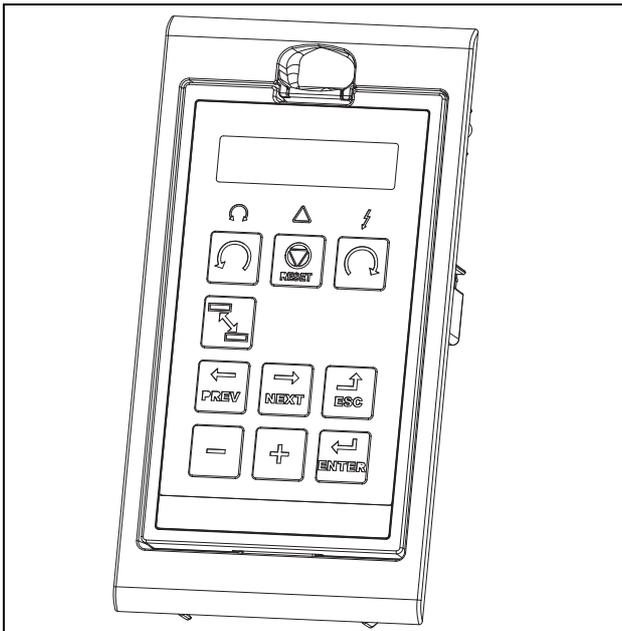
Fig. 55 Control panel in mounting cassette
