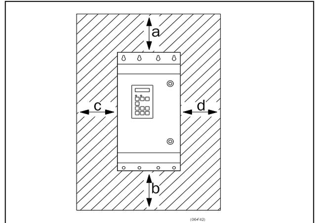
Fig. 3 AC drive mounting model 003 to 293
