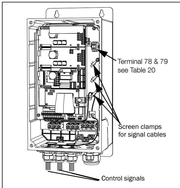
Fig. 42 Connecting the control signals, FLD model 003 to 018, frame size B.
