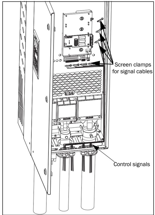
Fig. 47 Connecting the control signals, FLD model 48-090 to 295 and FLD model 69-90 to 200, frame size E, F and F69 (principle drawing).
