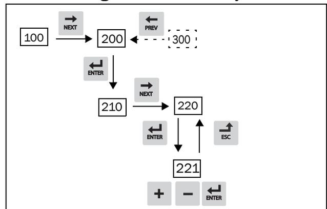
Fig. 50 Example of menu navigation when entering motor voltage
