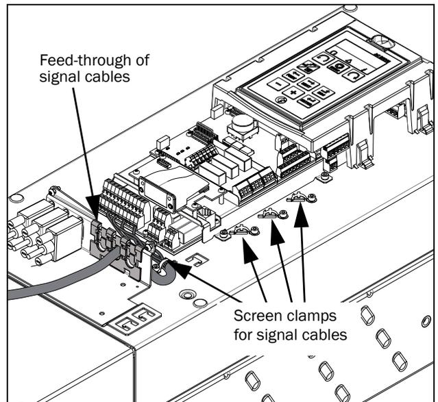
Fig. 48 Connecting the control signals, FLD model 48-142 to 48-293 frame size E2 and F2 (principle drawing)
