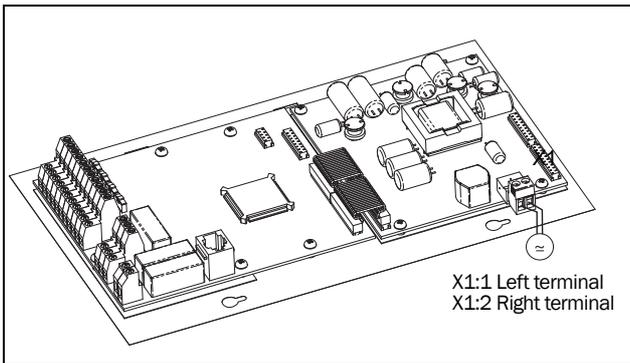
Fig. 56 Connection of standby supply option in frame sizes B, C, C2, E, E2, F and F2.
