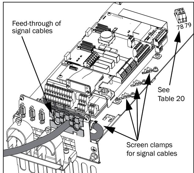
Fig. 44 Connecting the control signals, FLD model 48-025 to 48-058 frame size C2.
