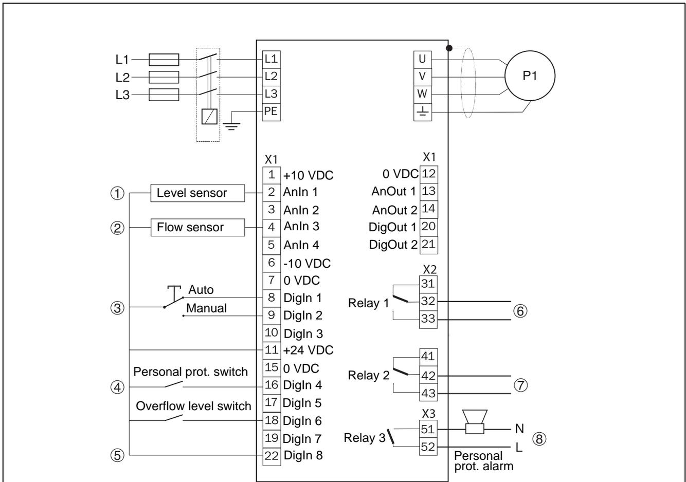
Fig. 40 FlowDrive standalone full wiring examples.
