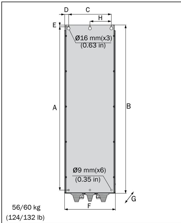
Fig. 15 Emotron FLD Model 48-090 to 175 (Frame size E).
