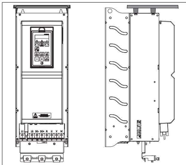
Fig. 61 Optional top cover mounted on frame size D2
