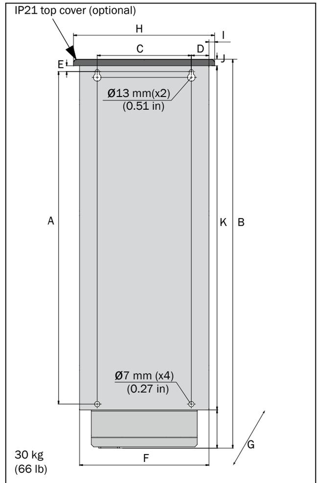
Fig. 13 Emotron FLD Model 48-072 to 48-088 (Frame size D2), backside view.
