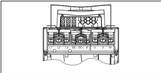
Fig. 20 Bottom view Emotron FLD Model 48-106 to 48-293 (Frame size E2 and F2), with cable interface for mains, motor, DC+/DC-, brake resistor and control. (principle drawing)
