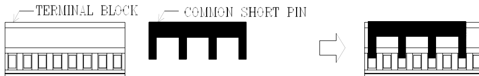
Terminal Block and Common Shorting Pin Assembly
