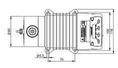
$Fig. \ 5: \ Dimensioned \ drawing \ of \ MAGDOS \ LA/LD \ with \ dosing \ head \ made \ of \ PVC, PP \ or \ PVDF \ (all \ dimensions \ in \ mm)$
