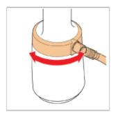
The 360° revolvable air supply unit can be turned in any position so that the hose does not obstruct your work space. Thus providing a comfortable and safe work environment.
