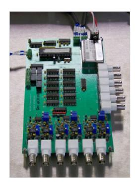
If a single detector input is used, the other amplifier/discriminator units can be configured to serve as single-channel amplifier/discriminators to provide region-of-interest count values for different energy signals. Thus, each input can either be connected to a separate detector or, by internal switch selection, can be linked to other inputs to provide selective counting of adjustable region-of-interest count scaling, for example for gamma-ray spectrum analysis.
