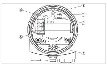
Oscillator - Contactless electronic switch
