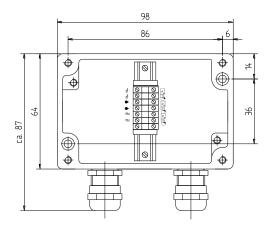
Cable glands which are not required have to be removed and the holes must be closed with the enclosed covers. With cable diameters of 4-8mm for load cells and 6-12mm for indicator connection, the cable glands and the housing reach up to protection class IP 65.
