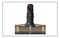
Terminator ZS/ZE...designed to fabricate accessible outside-the-insulation splices or end terminations of Thermon Heating Cables. Electrical connections are made using wire fasteners (for applications requiring terminations to be made with terminal block connections, the Terminator ZP kit may be used).
